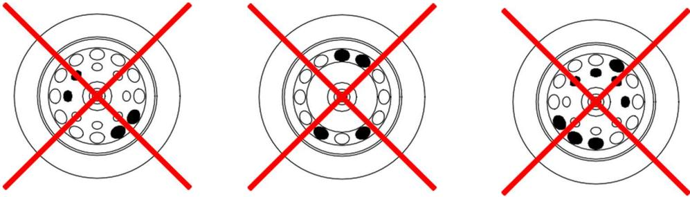
Incorrect loading examples for fixed angle rotor
