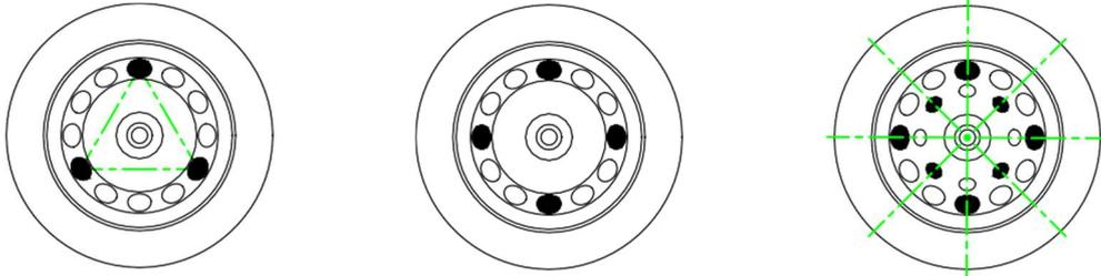
Correct loading examples for swing out rotors
